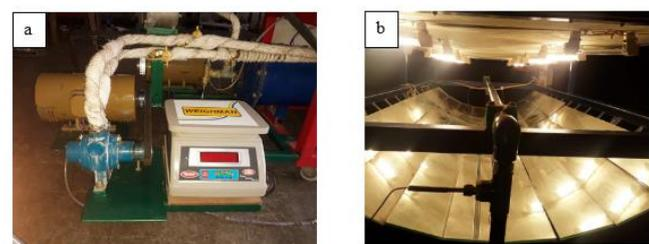
Figure 5: (a) Pump and weighing scale, (b) Parabolic trough collector
