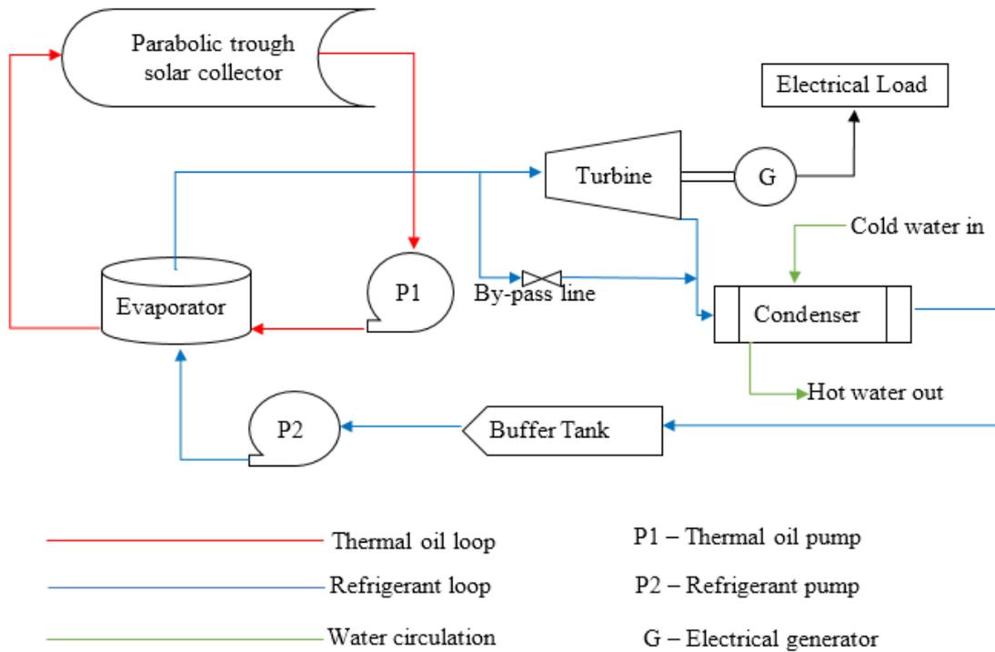
Figure 2: Outline of the ORC test setup
