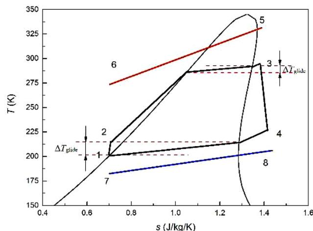
Figure 1: T-s diagram of general ORC
