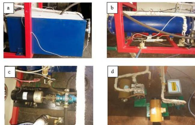
Figure 4: (a) Evaporator, (b) Condenser, (c) Thermic oil pump, (d) Expander with generator
