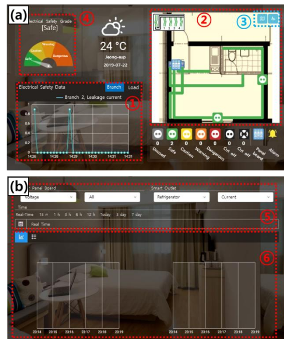
Figure 3. Configuration of the abnormal condition monitoring system of the electrical installation
