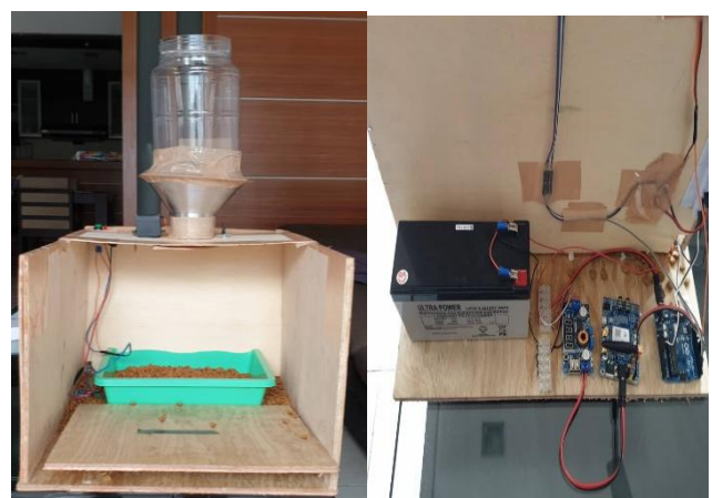
Figure 7: Front and back view of the smart pet feeding prototype
