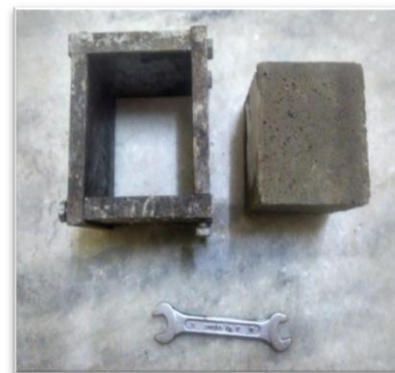
Fig.7 Cube after casting
