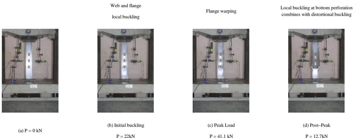
**Figure 6: Load-displacement progression for column SC103-1.2-A3**
