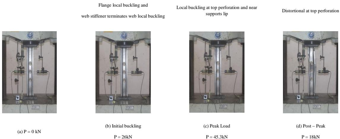
**Figure 7: Load-displacement progression for column SE103-1.2-A3**
