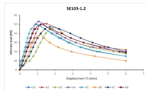
**Figure 4: Load-displacement curve for columns SE103-1.2**
