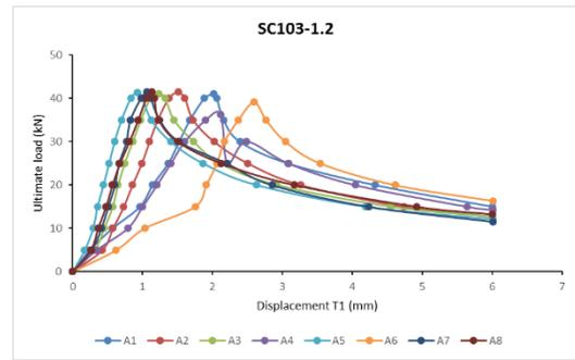
**Figure 4: Load-displacement curve for columns SC103-1.2**
