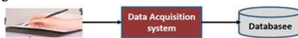
Fig 1. Block diagram of Data acquisition The pen patterns are stored in XML format which contains pen up and pen down information with file ID representing author, sample number.
