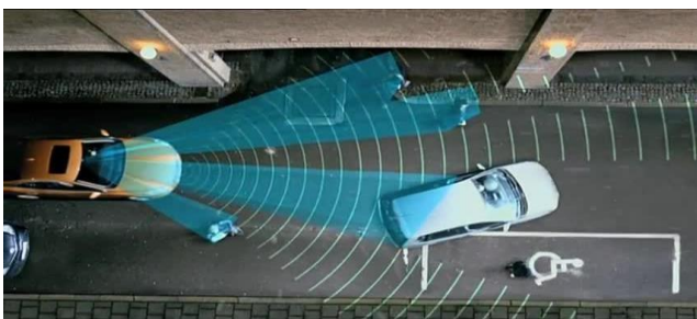
Fig. 2. The PAT system in a Volvo car detecting obstacles in each direction in front of it
