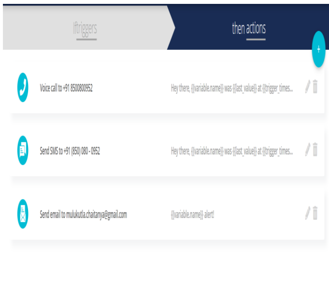
Figure 9. Ubidots actions done if event is triggered for switching OFF motor
