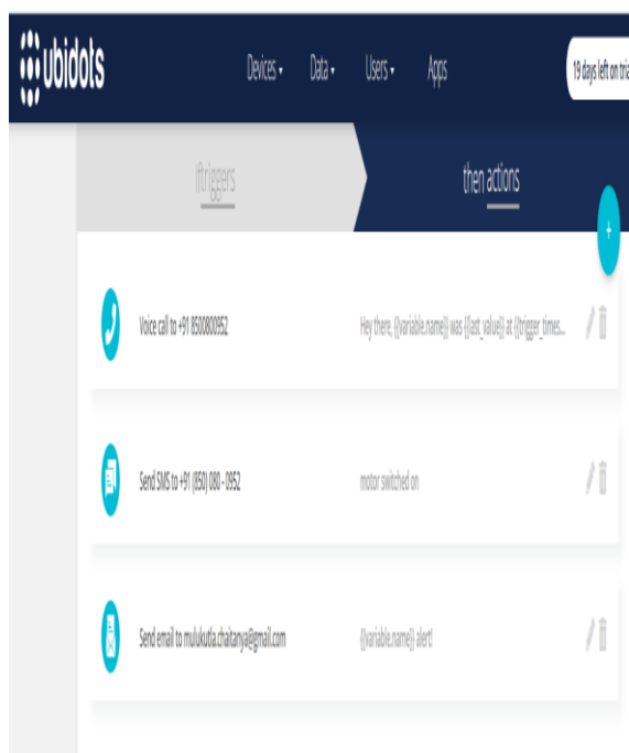
Figure 7. Ubidots actions done if event is triggered for switching ON motor
