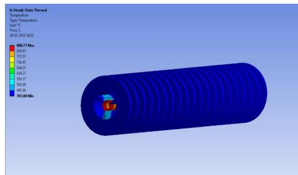
Fig. 2. Temperature distribution in helix-helix support rod assembly
