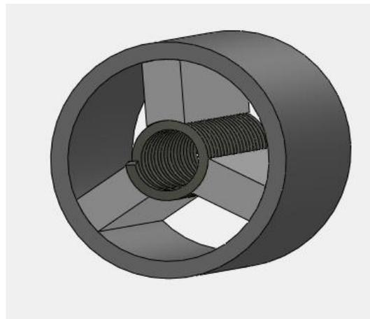
Fig. 1(a)3-D model of Helix support rod assembly
