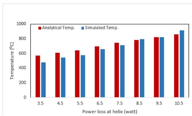
Fig. helix temperature at different power loss at helix
