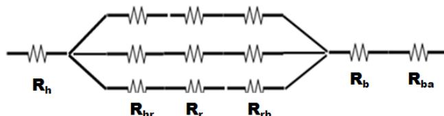
Fig. 1(b)Equivalent thermal resistance model for helix support rod assembly
