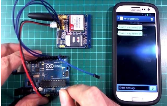
Figure 13: GSM & Arduino UNO Connectivity
