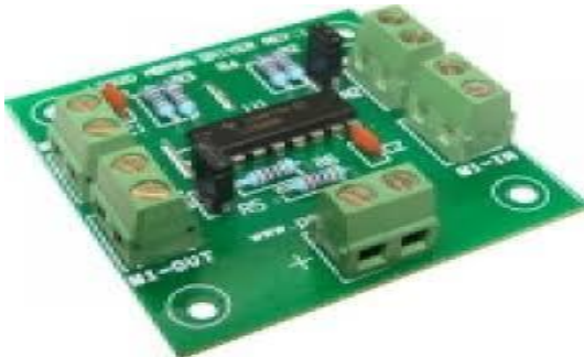
Figure 4: L293D H-Bridge IC
