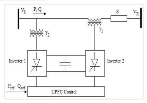
UFC costs of two voltage supply converters; Collection and shot converter, which is connected to each other with a dense DC link. The series converter or Static Syncona series is assigned to the voltage magnet day and chapter angle serial ser, while the stunt converter or static syncona component AC is assigned to provide responsive power System is made.
