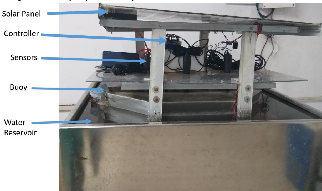
Figure 2. Buoy with Complete IoT setup
