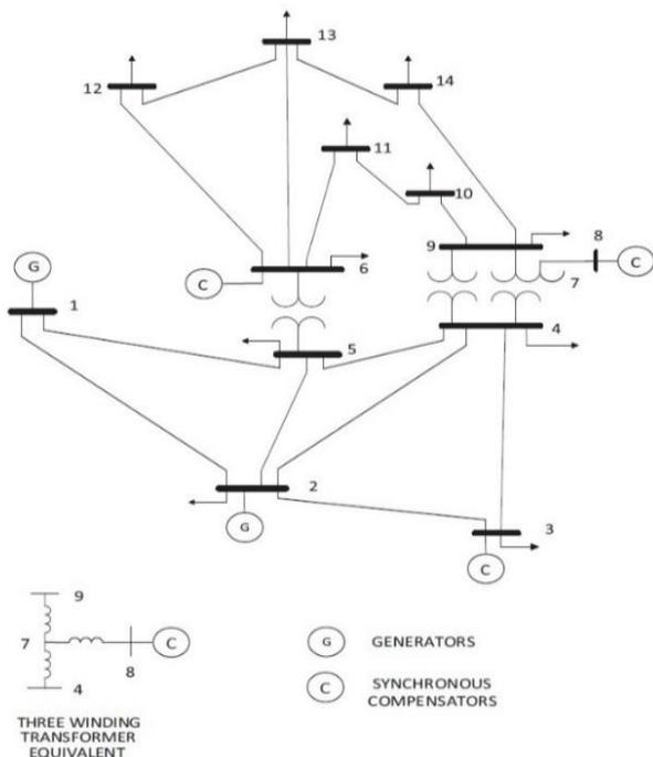
Fig. 1. IEEE 14-bus sub-transmission network
