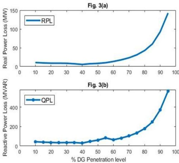
Fig. 3 (a-b). Characteristics of RPL and QPL for Type-4 DG with an increase in PL
