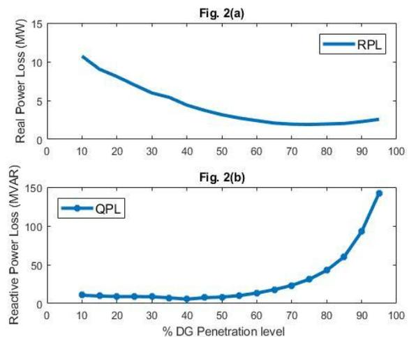
Fig. 2 (a-b). Characteristics of RPL and QPL for Type-2 DG with an increase in PL
