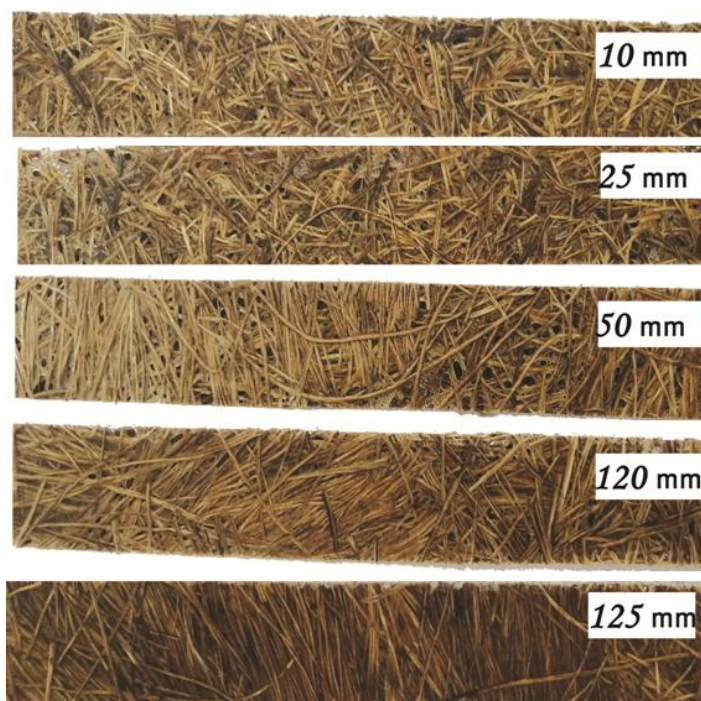
Fig. 2. Specimen for vibration analysis (10mm,25mm,50mm,100mm&125mm)
