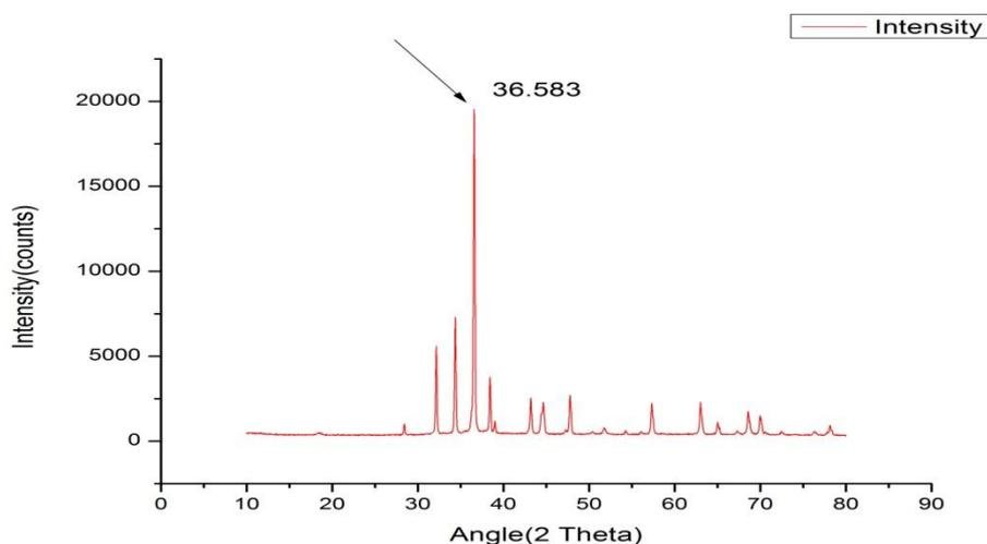
The XRD cerium pattern of Magnesium metal matrix is shown in Fig.1 The broad reflection seen at  $2\theta = 36.58^\circ$  shows nano reinforced properties present in the metal alloy
