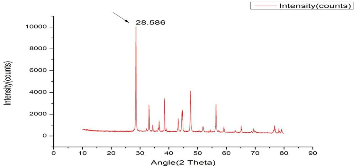
XRD pattern of Cerium dioxide doped lanthanum is shown in Fig.2 The broad reflection seen at  $2\theta = 28.58^\circ$  shows nano reinforced properties present in the metal matrix
