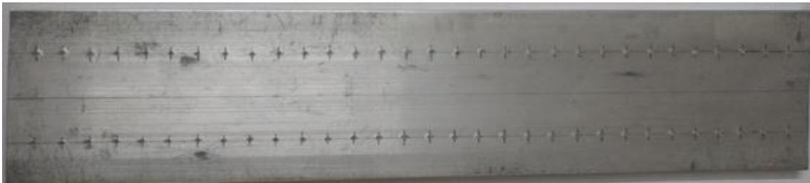
**Fig 1 Work Piece after drillingholes**
