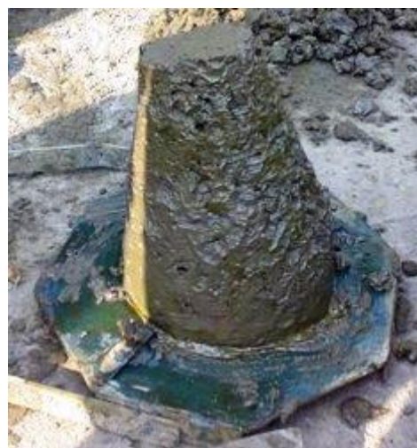
Fig 5.1 Slump Cone Apparatus
