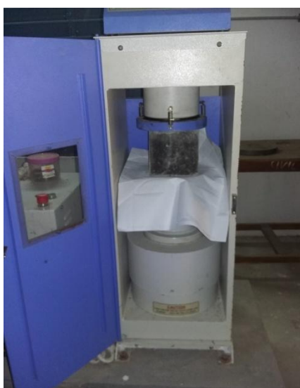
Fig 5.3 Cube placed on the CTM
