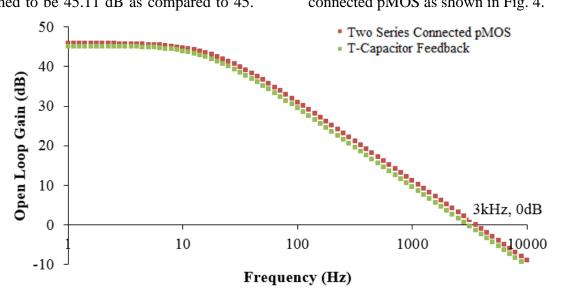
Fig. 4: Open-loop gain of Current Mirror OTA
