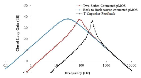
Fig. 5: Simulation results of closed-loop gain vs. frequency of Current Mirror OTA
