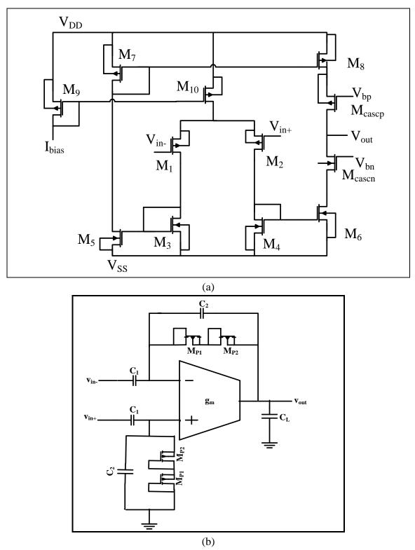
Fig. 1 (a) Current mirror topology for OTA (b) Closed Loop OTA with capacitive feedback [5]
