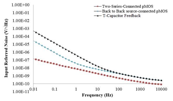
Fig. 6: Simulated input-referred voltage noise spectrum of Current Mirror OTA
