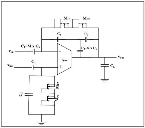
Fig. 2: Current Mirror OTA with T-capacitor feedback network [23]
