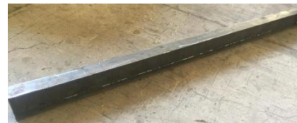
Fig. 11 : Beam with no stiffeners
