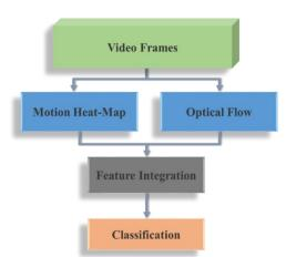
Figure 1:Flow diagram of Proposed Model
