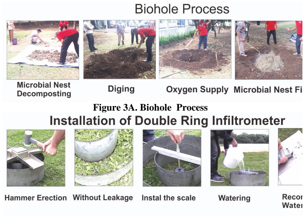
Figure 3A. Instalation of Doubel Ring Infitrometer
