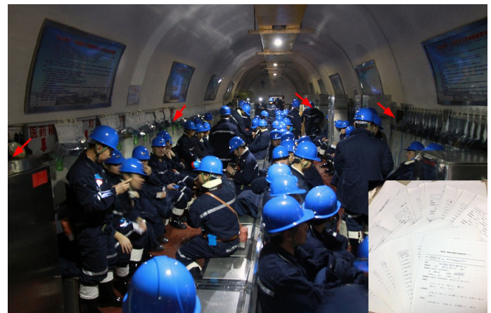
Fig. 9 On-site ventilation experiment and questionnaires (red arrows represented the positions of monitoring points).
