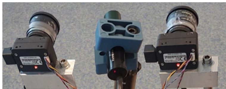
Figure. 7 The active stereovision system.
