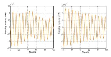
Fig. 6 Damping moment versus time using Eqn. (13). Left: Linear damping with wave exciting moment. Right: Linear damping without wave *Published by: The Mattingley Publishing Co., Inc.*
