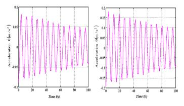
Fig.4 Acceleration versus time. Left: Linear damping with wave exciting moment(Eqn. (8)).
