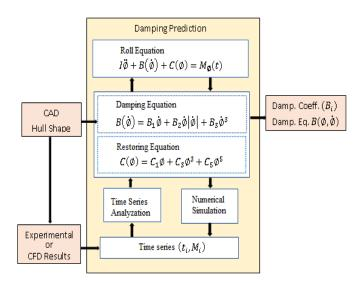
Fig. 1.Design of the roll damping prediction system
