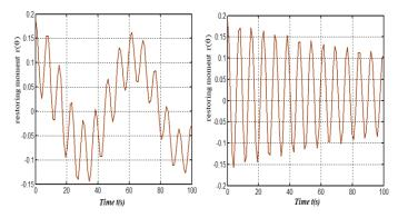
Fig.5 Restoring moment versus time Eqn. (12). Left: Linear damping with wave exciting moment. Right: Linear damping without wave exciting moment.
