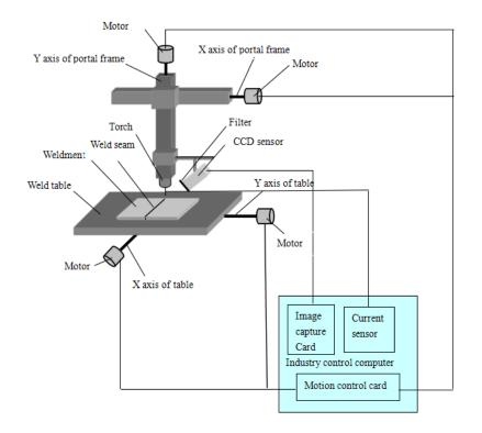
Fig.1. Welding Experimental System
