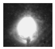
(b) Image filtering by neutral filterFig.2. Welding Images Filtering by Narrow Band and Neutral Filter
