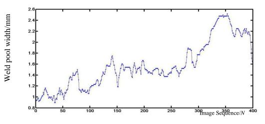
Fig.7. Weld Pool Width at the Back of Weld Seam
