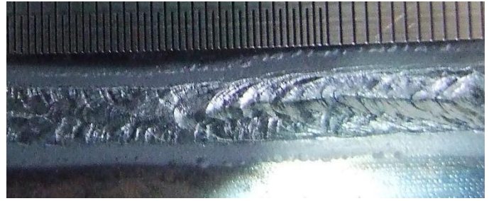
Fig.5. Front Side Image of Weld Seam after Welding Experiment
