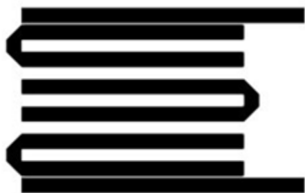
Figure 2: Microstrip Hairpin Structure[18]
