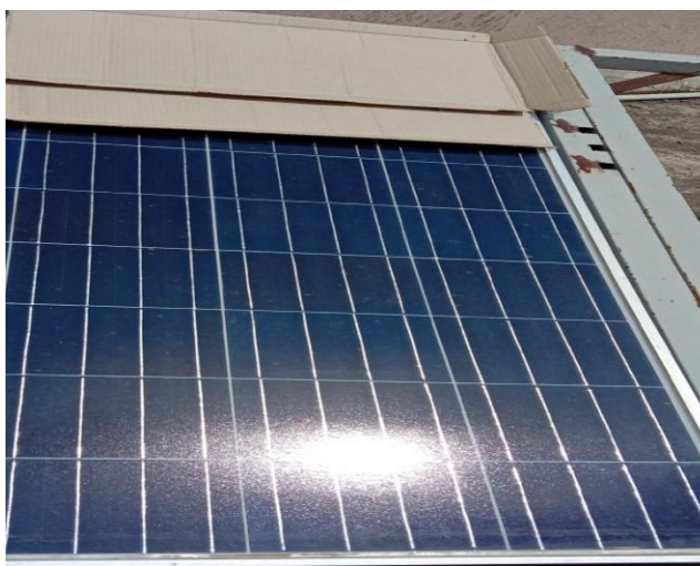
Fig 4. With 25% shadow on the panel created by cardboard
