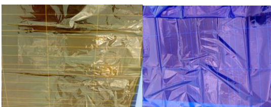
Fig 3, yellow and violet color filters wrapped on the panel
