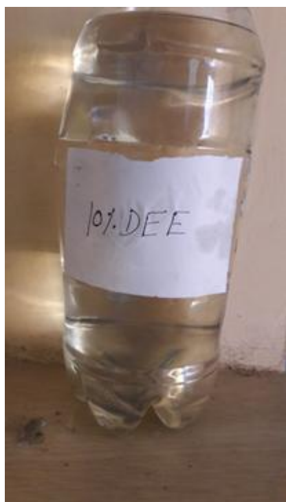
Figure 3 Arrangement of Diethyl ether and diesel in the wake of blending demonstrates no precipitation
