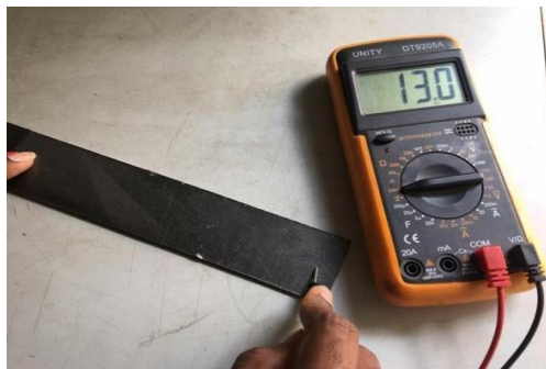
Fig6 Multimeter test probes at the ends of electrode
