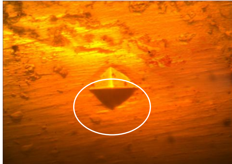
Fig. 4 Indentation image of coating produced under optimum condition
