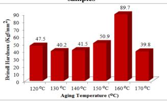
Figure 4: Brinell hardness of artificially aged 99.5Al-0.5Cr alloy
