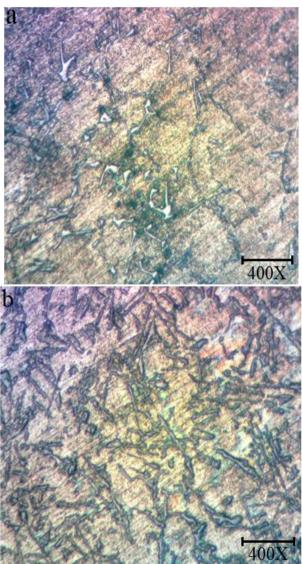
Figure 6: OPM micrograph of (a) Solution heat treated 99.5Al-0.5Cr alloy at 450 °C (b) artificially aged 99.5Al-0.5Cr alloy at 160 °C.
