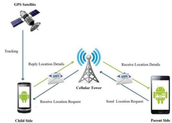
Fig 1: Architecture of Child Tracking System Using Android Phone
