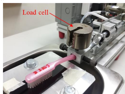
Figure 1. Reciprocating toothbrush simulator apparatus.
