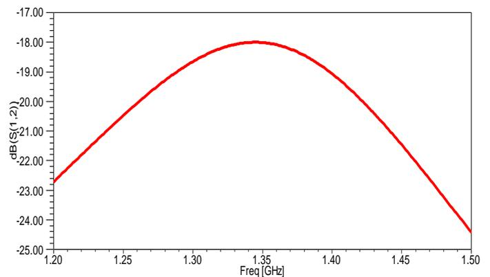
Figure 8. Mutual Coupling of the antenna array
