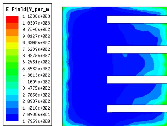
Figure 5. Current distribution at 1.35GHz
