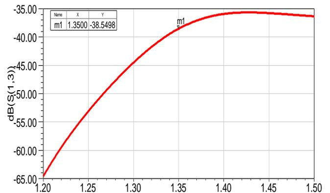
Figure 12. Mutual Coupling of the antenna array with EBG
