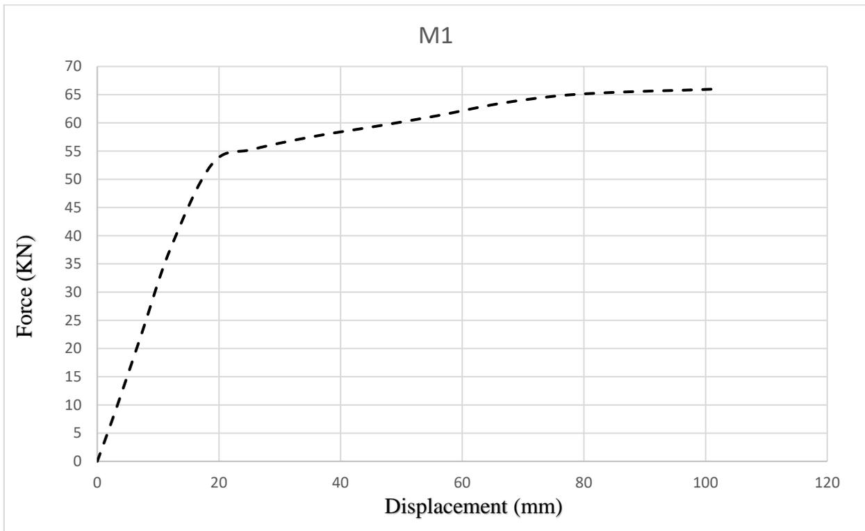
Fig 8: The Force-Displacement diagram of the M1 corrugated web beam.
