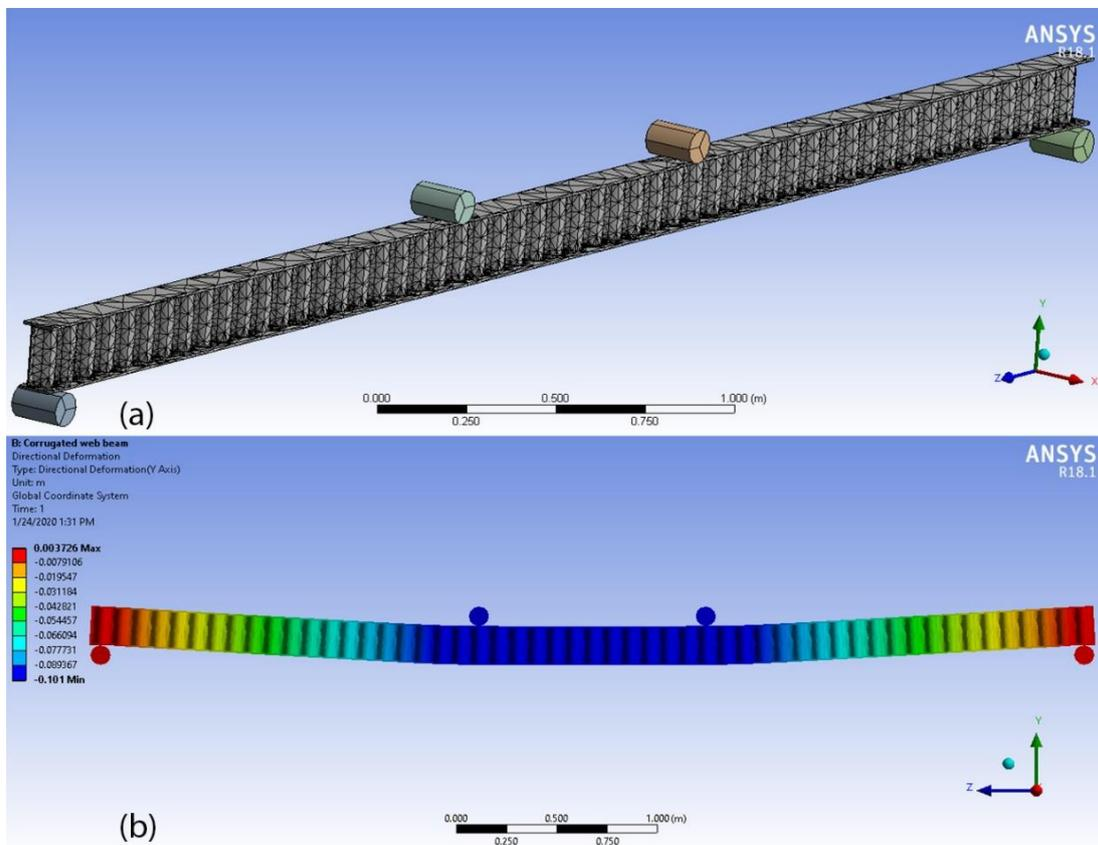
Fig 2: (a) the mesh used in the analysis (b) the deformed shape of the beam.
