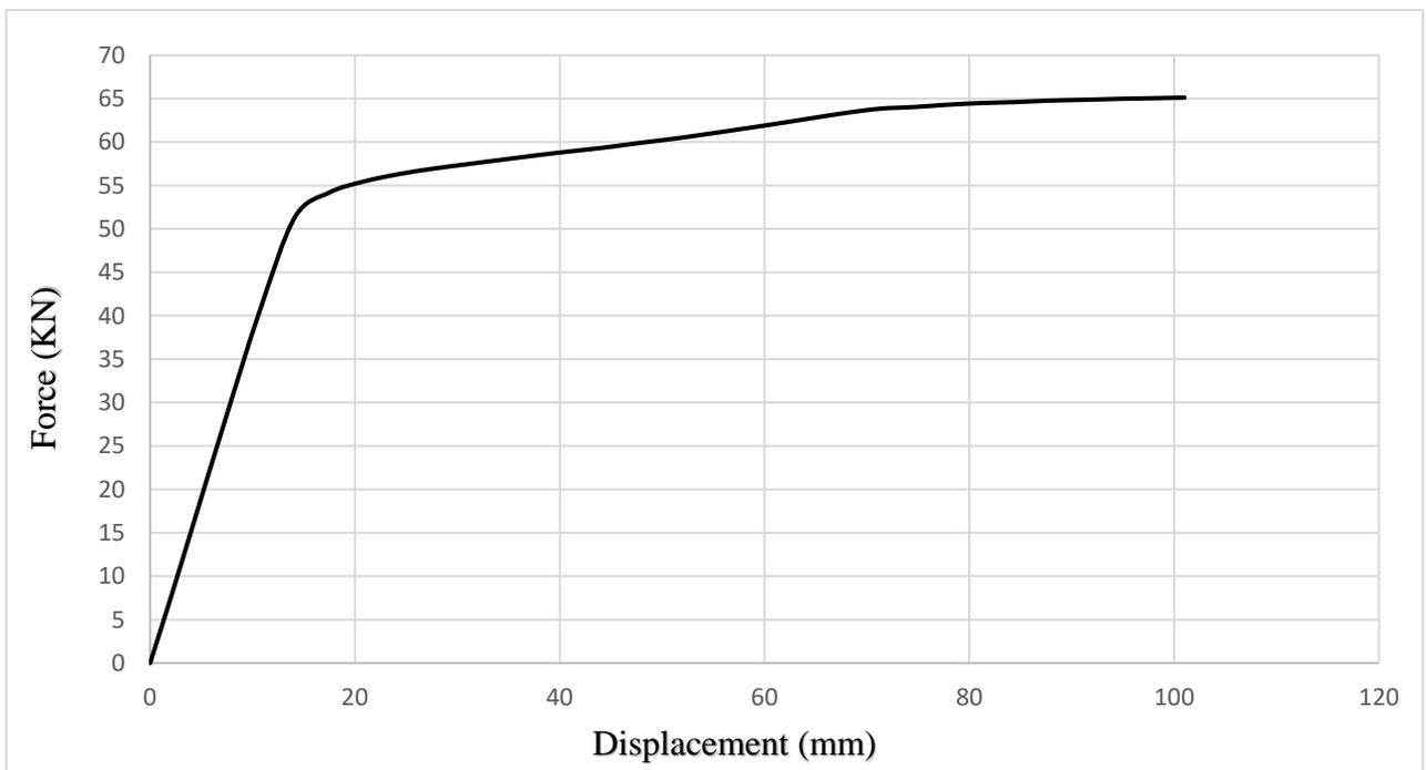
Fig 7: The Force-Displacement diagram of the original corrugated web beam.
