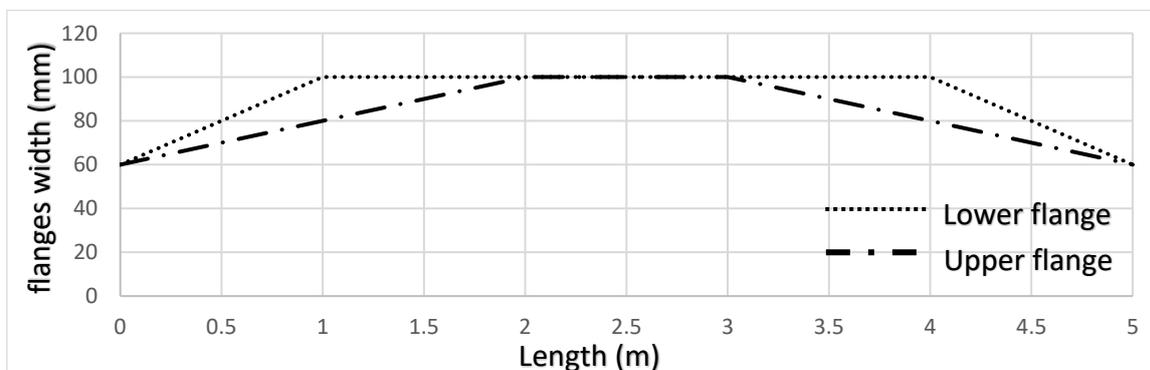
Fig 5: The width of the upper and lower flanges profiles of model (M3).
