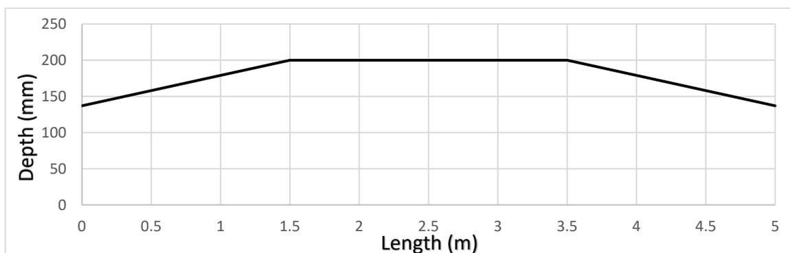
Fig 4: (a) The depth profile of the beam (M2) along its length.
