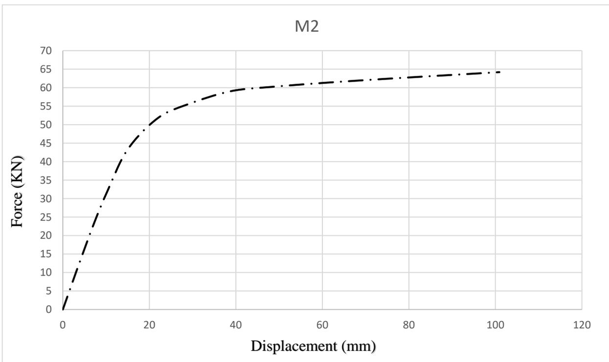
Fig 9: The Force-Displacement diagram of the M2 corrugated web beam.
