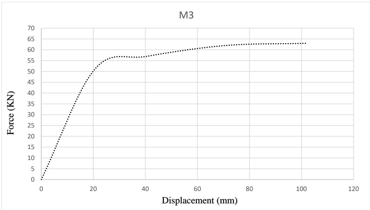
Fig 10: The Force-Displacement diagram of the M3 corrugated web beam.
