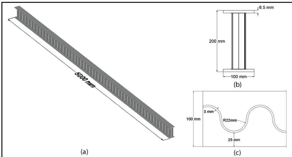
Fig 1: (a) 3D model of the corrugated web beam (b) the cross section of the corrugated web beam (c) the corrugated web.
