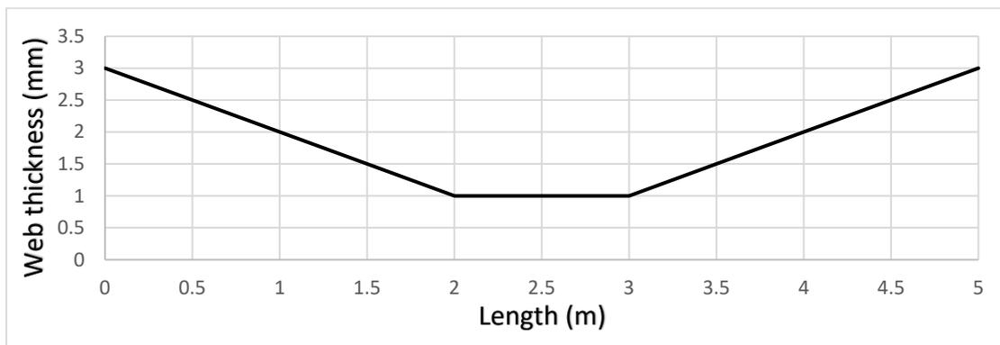
Fig 3: The thickness of web profile of the beam (M1) along its length .
